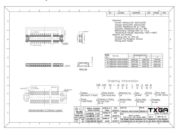
Figure 4: WisConnector PCB footprint and recommendations
