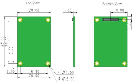
Figure 3: Mechanical Dimensions
