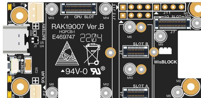
Figure 1: WisBlock Base Board 2nd Gen top view
