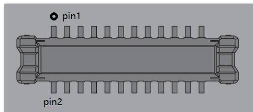
Figure 10: WisBlock Sensor module connector
