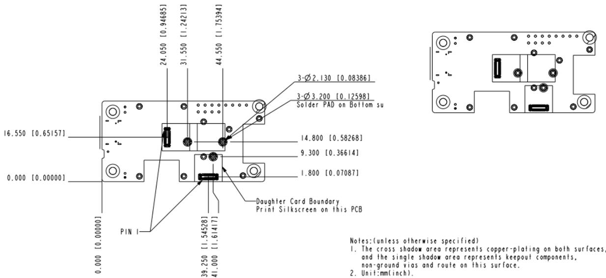
Figure 13: RAK19007 mounting holes location and diameter bottom view
