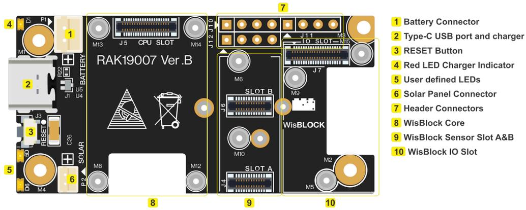
Figure 4: RAK19007 top view components
