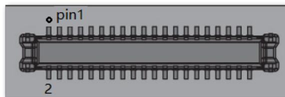
Figure 9: WisBlock Core module connector
