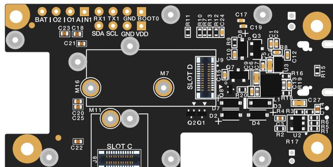
Figure 2: WisBlock Base Board 2nd Gen bottom view
