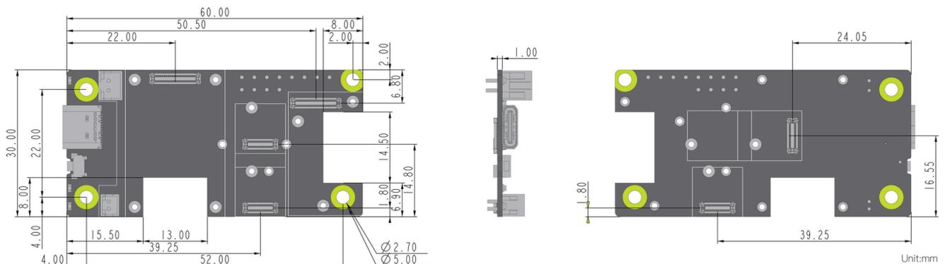
Figure 11: RAK19007 mechanical dimensions
