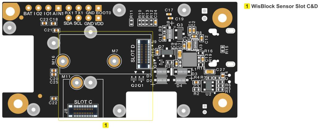
Figure 5: RAK19007 bottom view components
