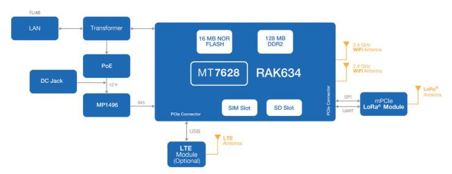
Figure 1: WisGate Edge Lite 2 Block Diagram
