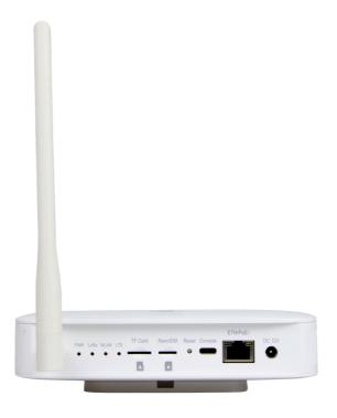
Figure 2: WisGate Edge Lite 2 Interfaces
